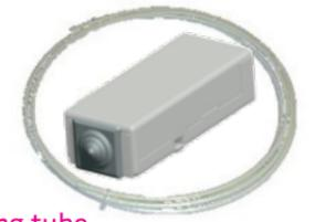
The BEM Cable Clamp is used to anchor the cable within the rack or to an SRS4000 Mounting Chassis and route the fibres onto the Modules. The BEM is suitable for cables between 36 and 192 fibres. 20 metres of routing tube is supplied with the BEM.
