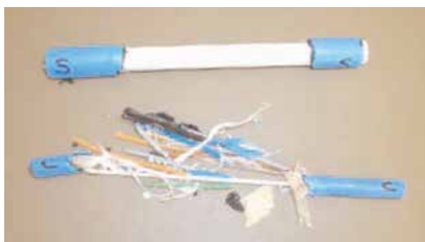
Rodent attack comparison: Severest attack examples. ARM@CORE (S) vs. Conventional Loose Tube Cable (C)
