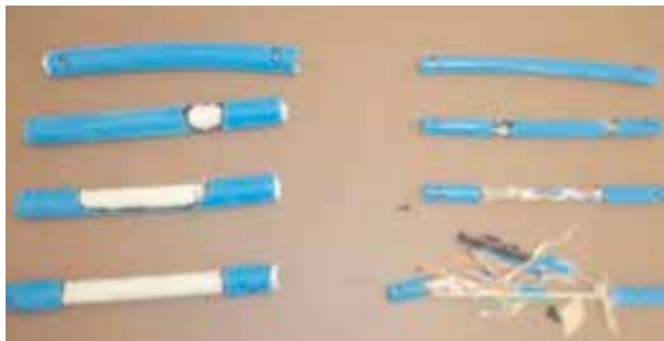
Stages of Rodent attack damage from day 1 (top) to day 7 (bottom) ARM@CORE (S) vs. Conventional Loose Tube Cable (C)
